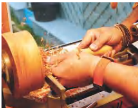
▲ The short length allows easy access without removing the headstock
